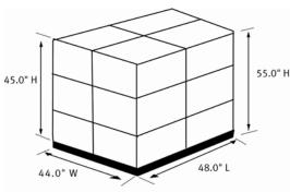
12 Boxes in a pallet NOTE: Actual pallet measurement is 48" L x 44" W
